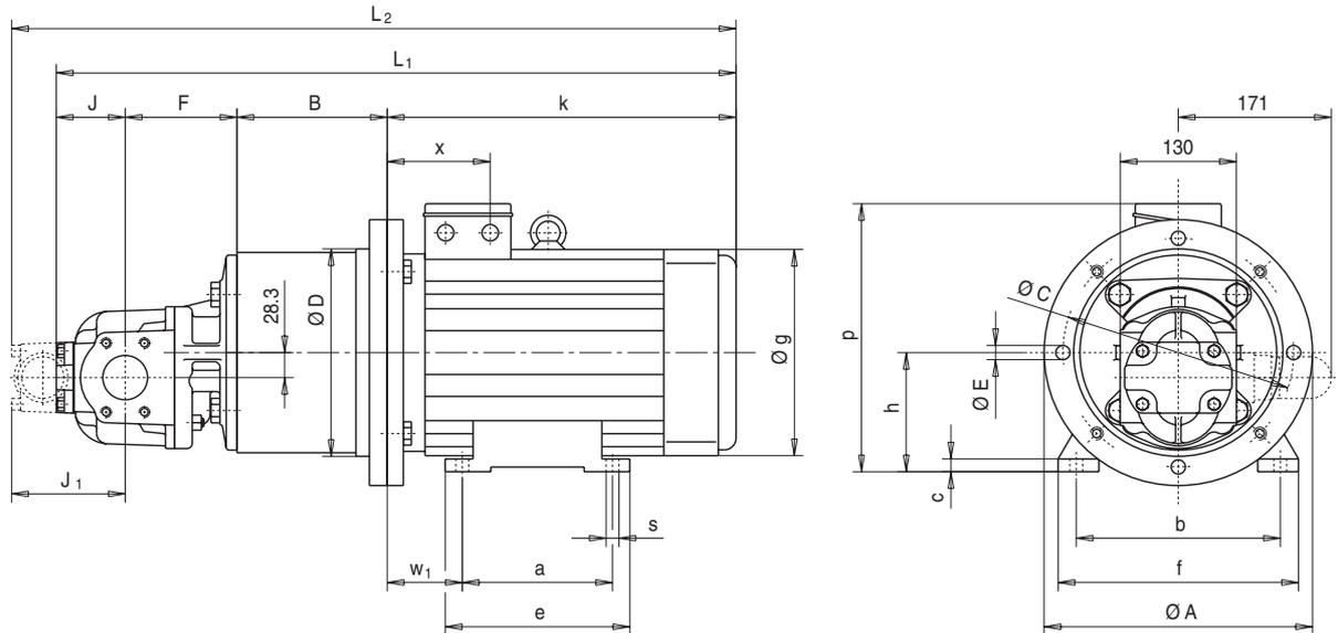
Motorbauform: IM B35 (IM V15; IM V36)
