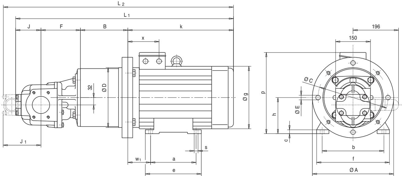
Motorbauform: IM B35 (IM V15; IM V36)
